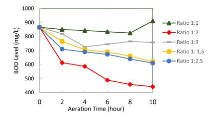
Figure 3. BOD level Vs Aeration time
