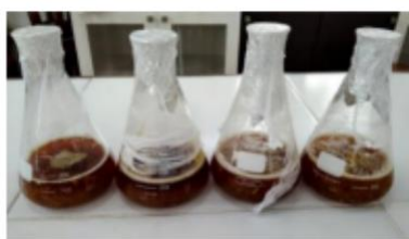
Figure 1. Color of corn husk powder during delignification
