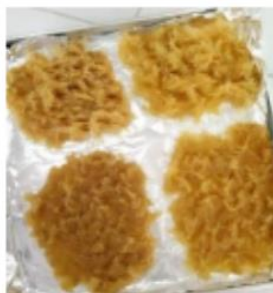
Figure 2. Color of corn husk powder after delignification
