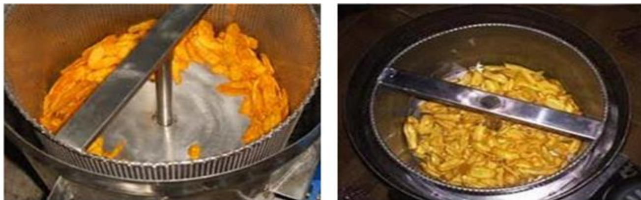
Figure 3. Draining oil with a spinner.
