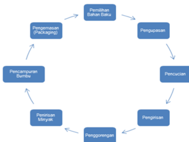
Figure 1. The process of producing cassava chips.
