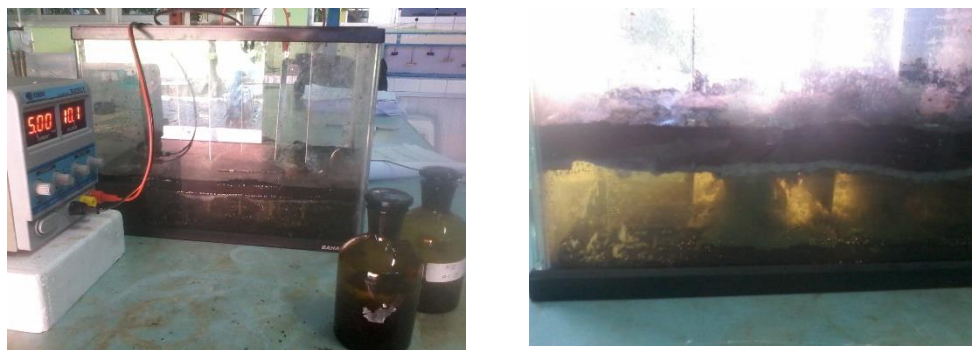
Figure 2. Bubbles binding the organic material forming the floc and bringing it towards the surface.
