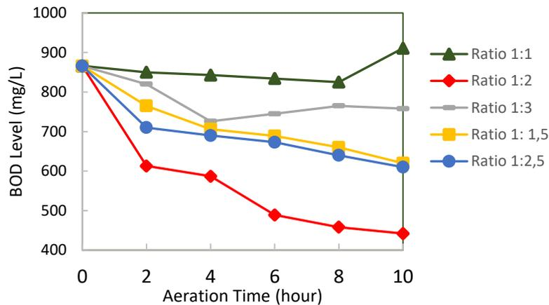
Figure 3. BOD level Vs Aeration time
