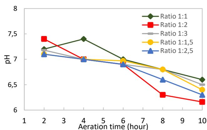
Figure 5. The pH versus aeration time on the sludge and wastewater from the crackers factory.
