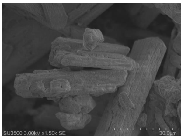
Figure 3. SEM analysis of struvite precipitation at pH 9.5 at temperature 35°C
