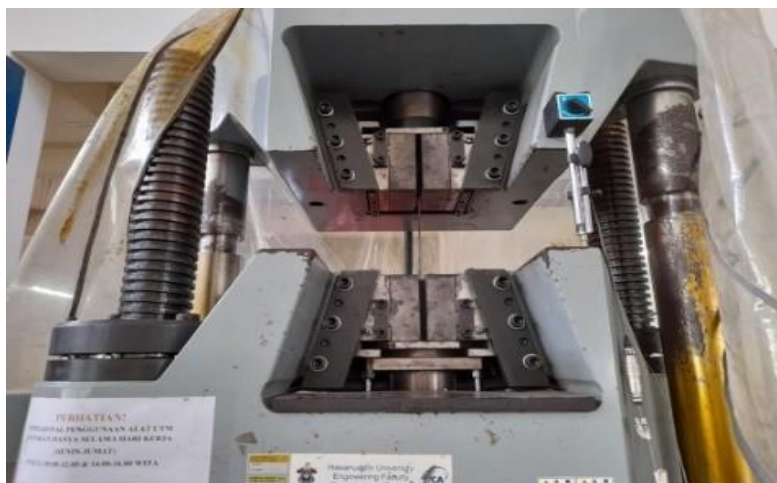
Figure 2. Tensile testing with Universal Testing Machine (UTM) 1000 KN capacity
