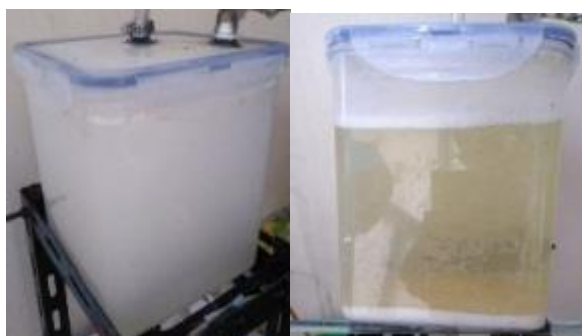
Figure 6. Saturated electrolyte solution and precipitation after electrolysis
