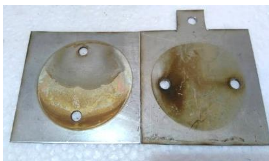
Figure 4. Residual catalyst on electrode
